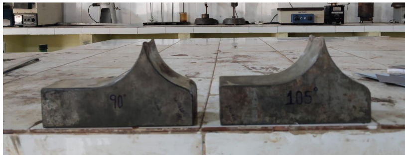
Fig.6: ECAR dies with 90° & 105° angles
