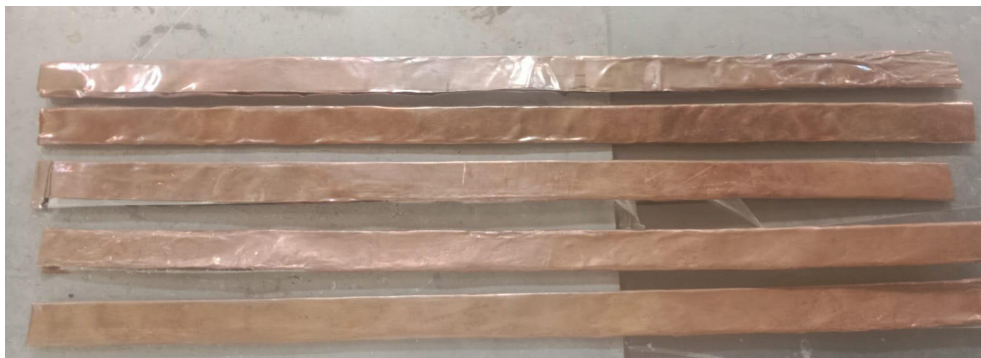
Fig.5: AA5083 samples with copper shielding before ECAR
