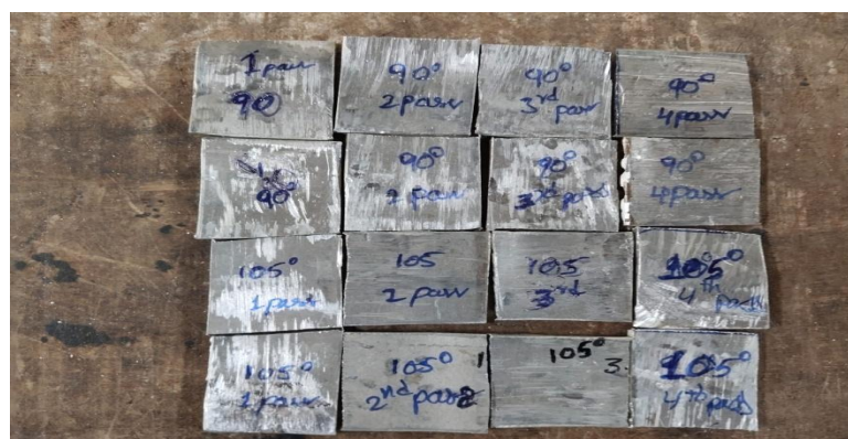
Fig.9: Samples for Microstructural Analysis after different passes
