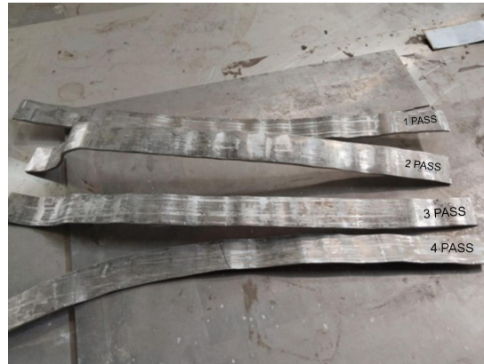
Fig.8: AA5083 Without Copper Shielding processed through 90° die angle
